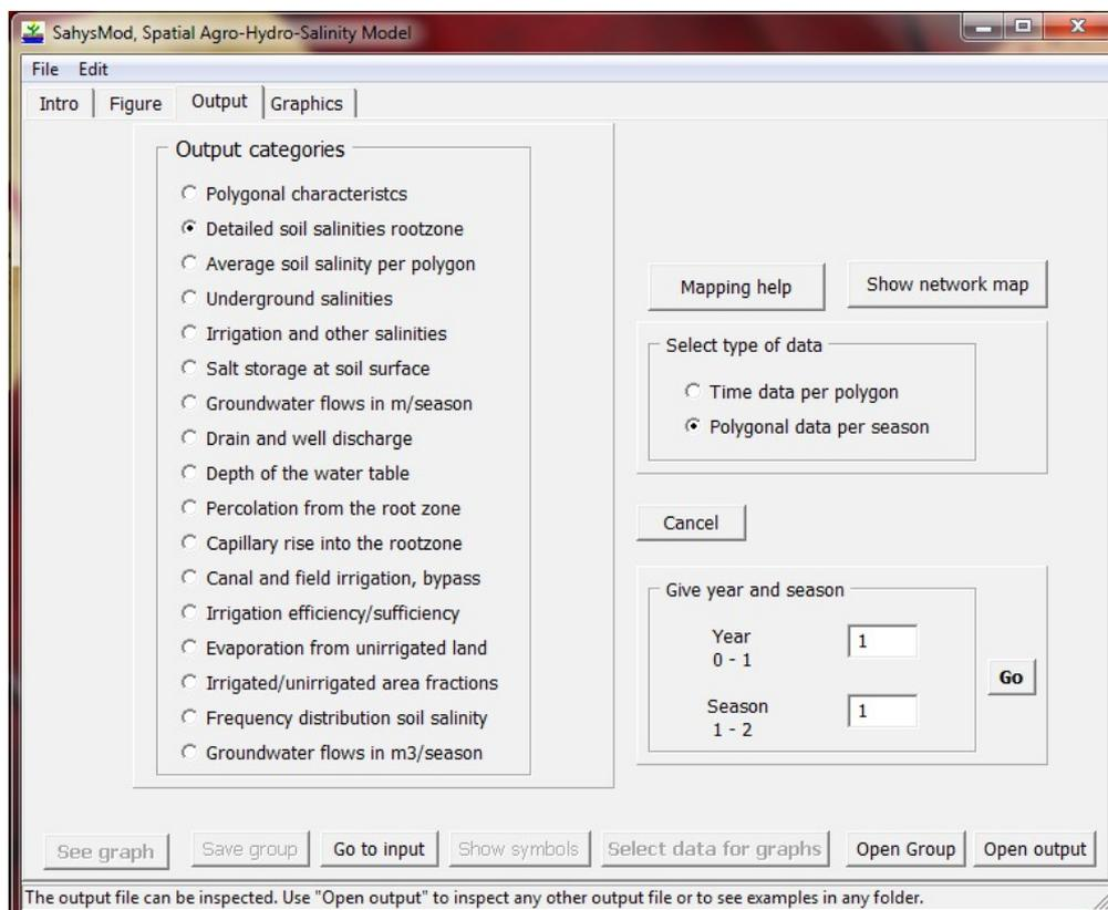
**Figure 1. Output categories of Sahysmod and output selection procedure.**
