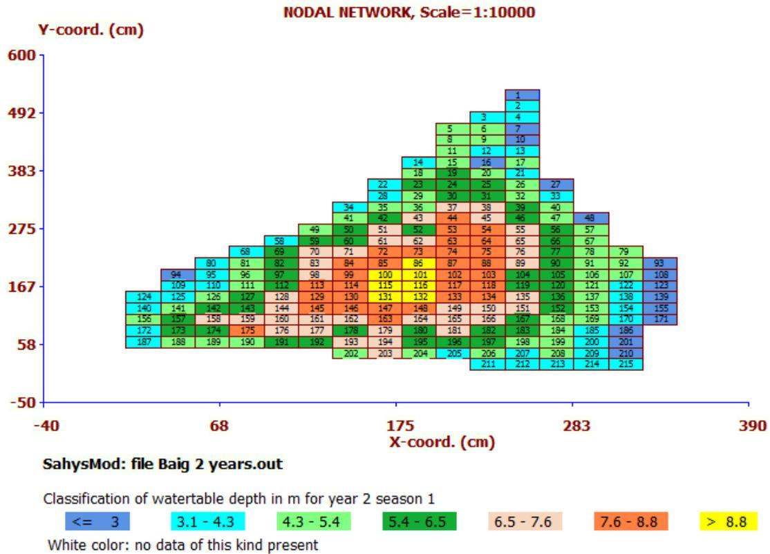
**Figure 13.** The water table is fairly deep except in the dark blue polygons bordering the river. Especially the central part of the region has deep water tables. This may be partly due to the scarcity of irrigation water as discussed before so that the recharge to the water table is limited.
