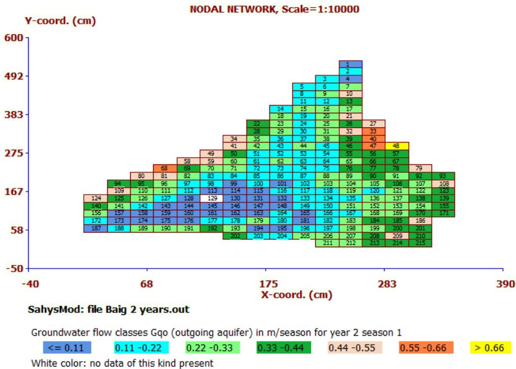
**Figure 11.** Groundwater outflow through the aquifer per polygon. The inflow (figure 10) reduced by the outflow (this picture) determines the depth of the water table, together with other water balance factors like downward percolation and upward capillary rise.
