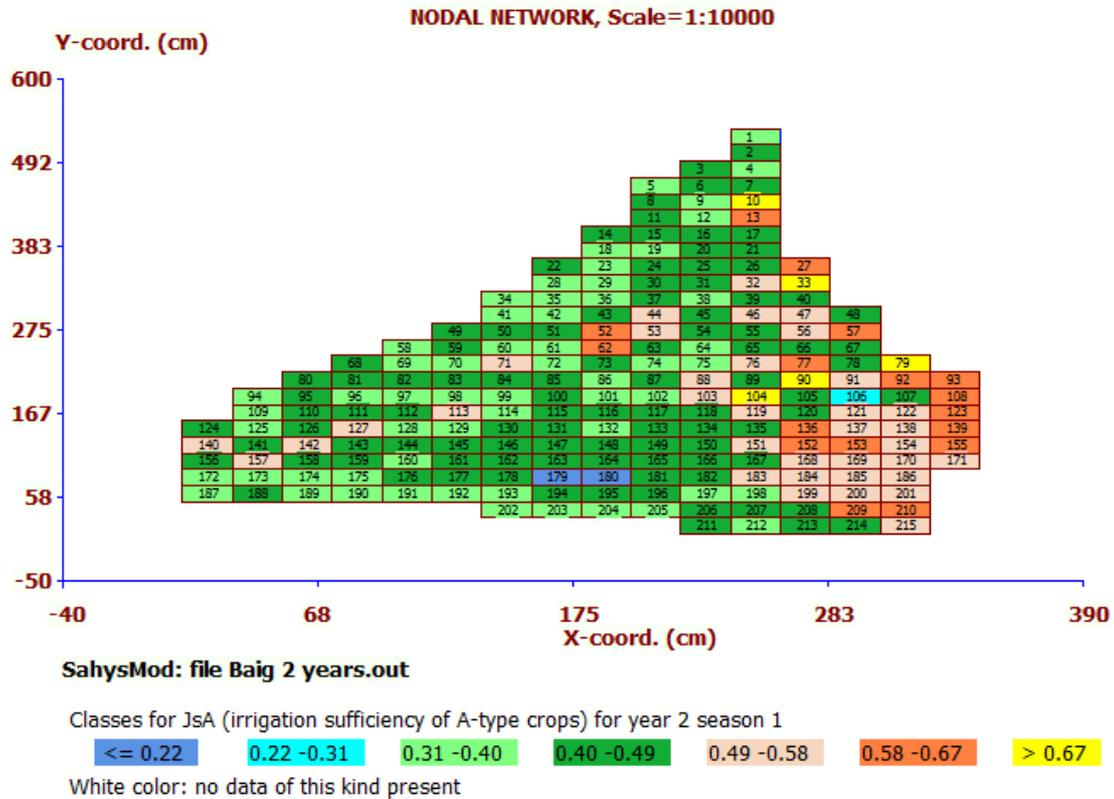
**Figure 12.** This makes it clear that the irrigation sufficiency is low and that scarcity of irrigation water plays an important role in the region
