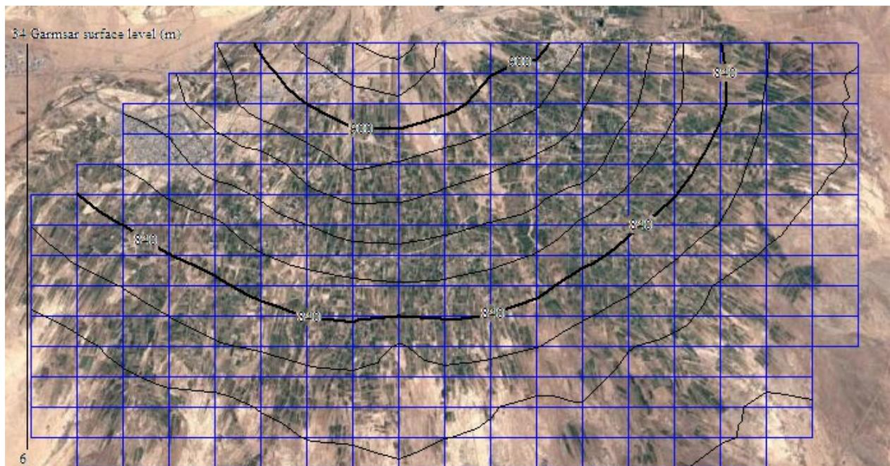
The Garmsar alluvial fan (Google Earth) overlain by the SahysMod nodal network (blue lines) and the surface level contour lines (black) made with the QuikGrid program, see <https://www.waterlog.info/pdf/QuikgridHelp.pdf>.
